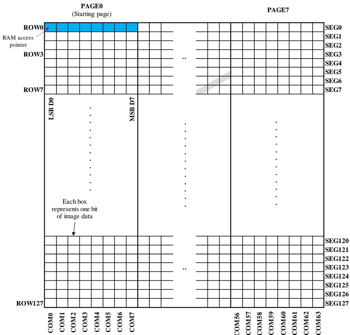
**Figure 2-4 : GDDRAM access pointer setting and orientation (No row and column-remapping) in SEG-Page Mode**
