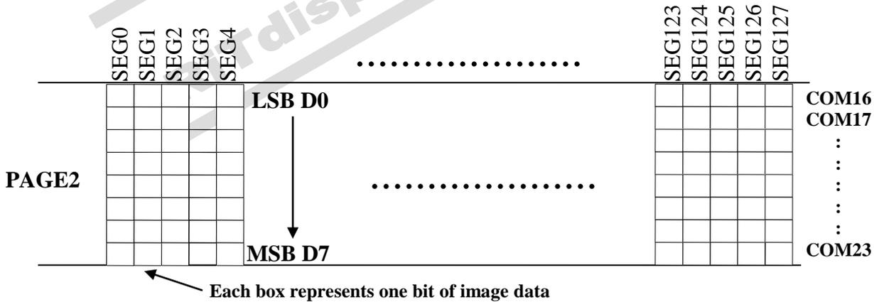
For mechanical flexibility, re-mapping on both Segment and Common outputs can be selected by software as shown in **Figure 6-13**.
