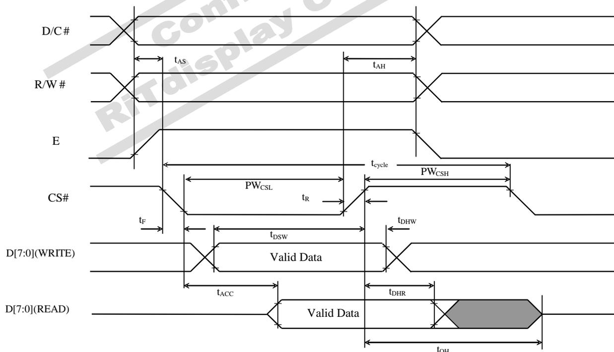
**Table 9-3: 8080-Series MCU Parallel Interface Timing Characteristics**
