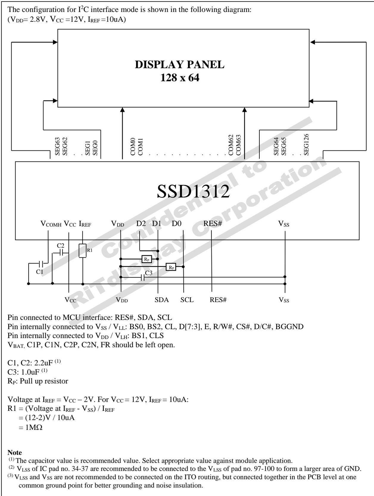
**Figure 10-2: Application Example of SSD1312 with Internal Charge Pump and I<sup>2</sup>C interface**
