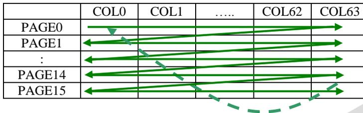
In normal display data RAM read or write in COM-Page or SEG-Page mode, the following steps are required to define the RAM access pointer location:
